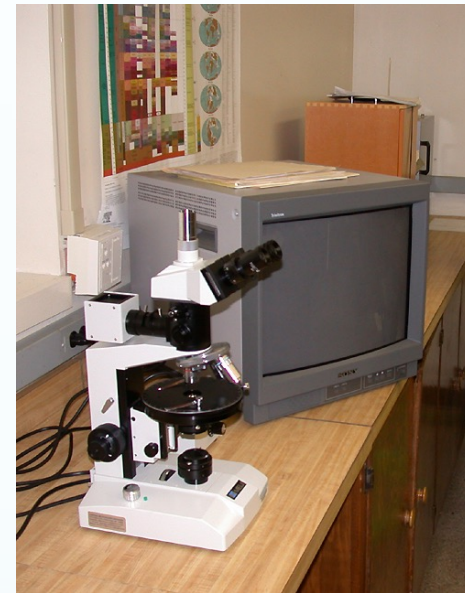
New petrographic microscope With digital camera and monitor
